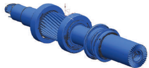
Re-engineered pinion of geared turbine, solving problem of thrust fixating after troubleshooting.
